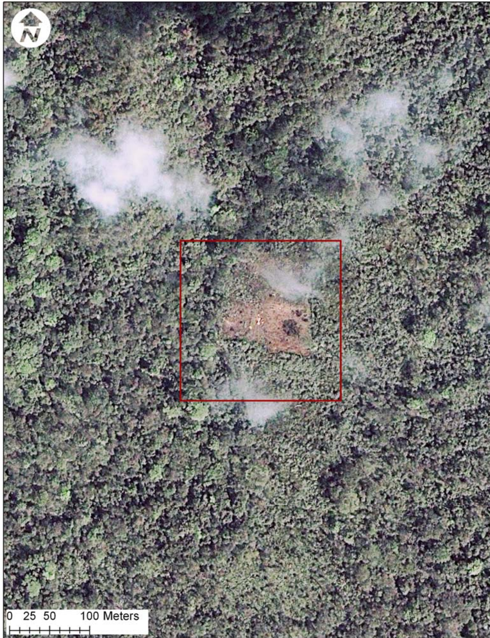
(Figure 4) Pan sharpened IKONOS RGB/ 321 from 2007. Resolution of the IKONOS at 1:3,749. The area of the red box is 200 square meters. Note the ability to see the structures and variation of the cleared areas.
